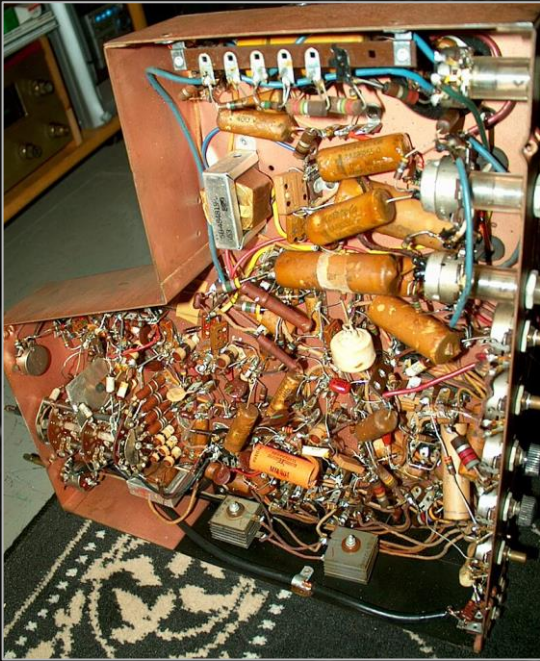
Point to Point wiring on a chassis
