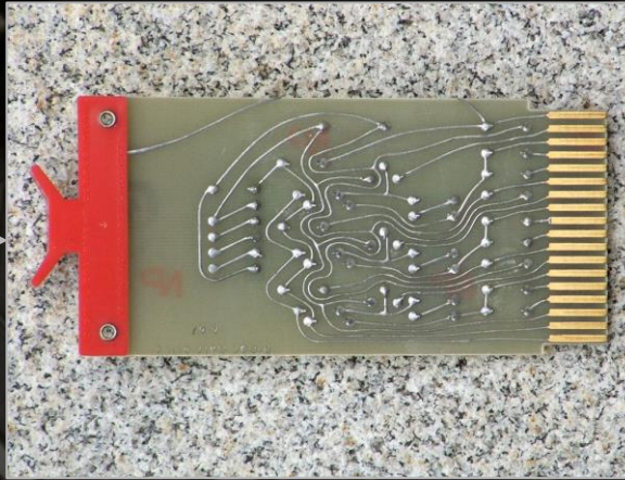
Drawing traces by hand and etching
